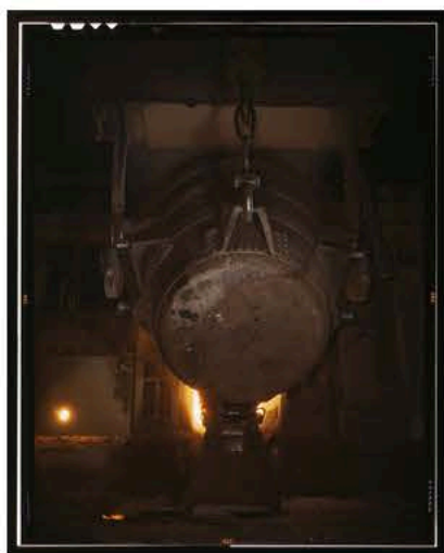
Ladle of molten iron is poured into an open hearth furnace for conversion into steel...
